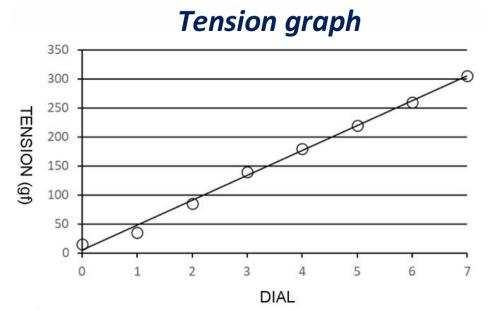
Tension data varies with yarn size and speed. This chart was compiled using 500 filament Polyester yarn at 36m/min speed.
